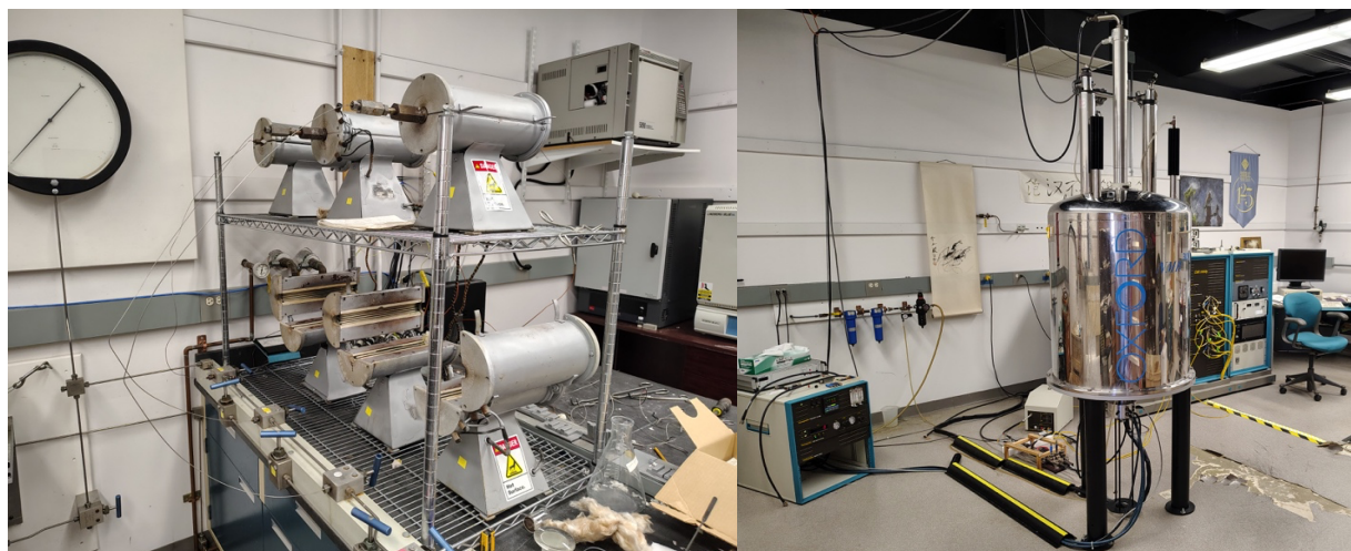
Figure 2: (Left) Hydrothermal reaction vessels. Each sample was placed in a silver reaction capsule, then enclosed in a reaction vessel before being heated in a furnace with a thermocouple. (Right) The ssNMR instrument that is being used to analyze MOM products. NMR analysis is ongoing and will reveal MOM molecular evolution.
